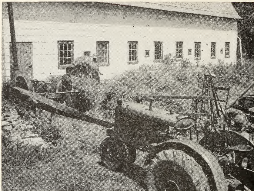
FIGURE 23.—In stationary chopping the material may be buckraked to the stationary chopper and pitched by hand into the chopper, which is ordinarily a standard ensilage cutter adjusted to handle hay. If the bucking distance is short enough, two men are required to handle the hay at the chopper. A two-man crew ordinarily chopped slightly more than 1 ton of hay per hour by this method.
